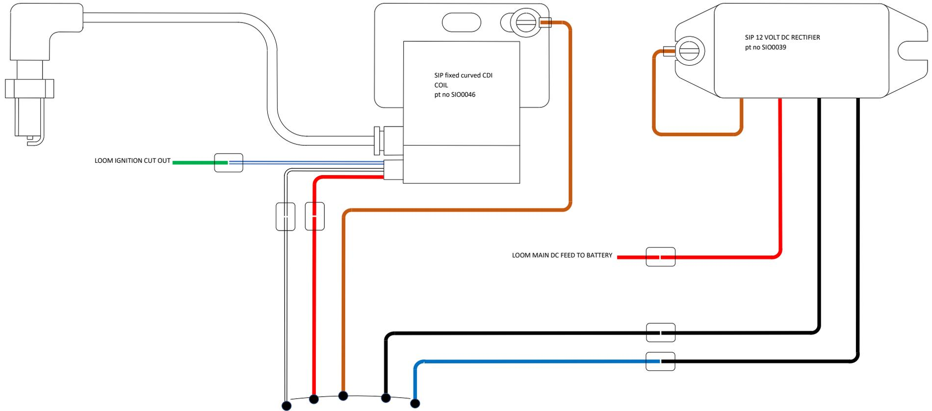
MB way... to bring the Vape DC inline with normal Lambretta colour coding - wire direct with connectors, don't bother using the spares and extra wiring that comes in the kit
