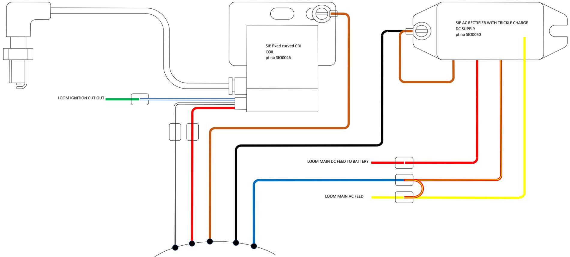
MB way... to bring the Vape AC with DC trickle charge inline with normal Lambretta colour coding - wire direct with connectors don't bother using the spares and extra wiring that comes in the kit
