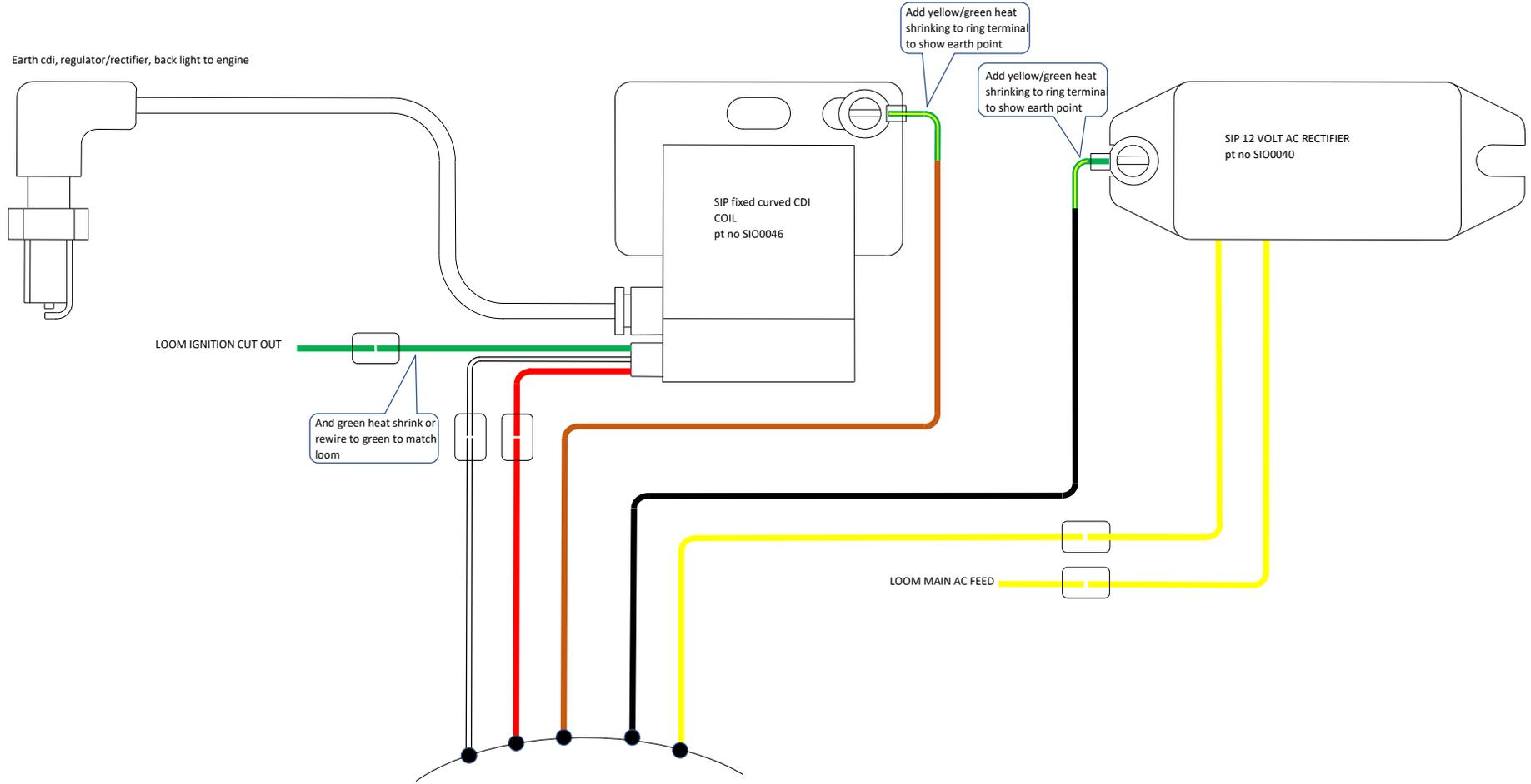
Vape DC wiring as per instructions, wire direct with connectors don't bother using the spares and extra wiring that comes in the kit
