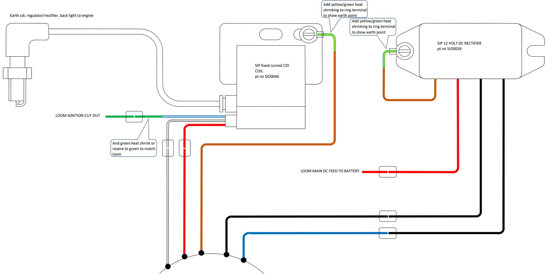
Vape AC with DC trickle charge wiring as per instructions, wire direct with connectors don't bother using the spares and extra wiring that comes in the kit
