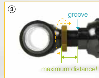
3) groove has to be covered completely in shocker mainbody
