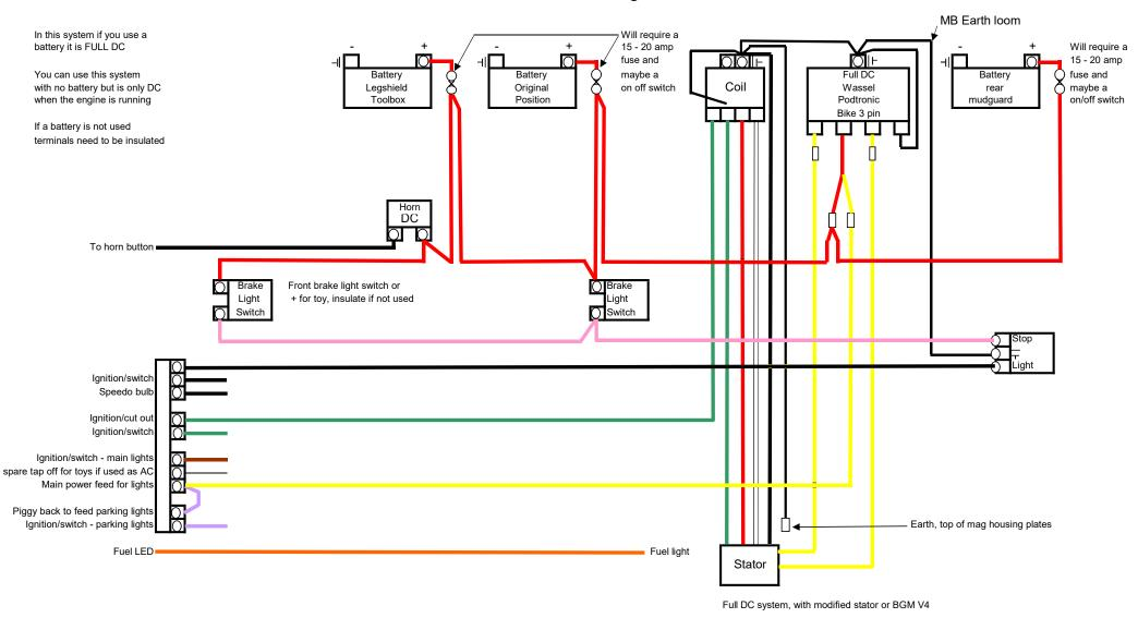
MB SERIOUS OUTDOORS SIMPLE AC or AC/DC or FULL DC WIRING LOOM Copy right Mark Broadhurst 26.1.13
