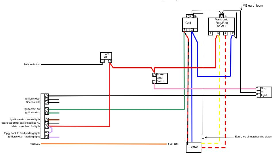
ELECTRONIC WIRING LOOM - VARITRONIC AC only using MB Looms MRB0803K/MRB0804K
