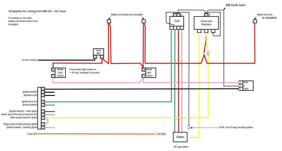
MB, SIL, VESPA, AF electronic to replace old simple looms, 12 volt AC only using MB Looms MRB0803K/MRB0804K
